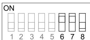
Figure 38: CDR-3 parity and baud rate settings
