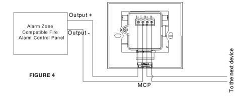
**NOTE**: Note: To operate correctly, the MCP must be connected to an Alarm Zone compatible fire alarm control panel (28VDC/60mA max.). Connecting the call point directly to 24VDC power may damage the MCP.
