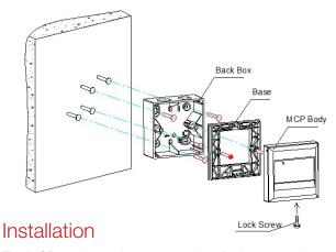
The MCP can be surface, recessed or flush mounted:
