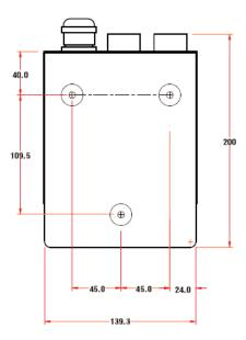
Leave 80mm clearance at top and bottom of docking station for access  $% \left( 1\right) =\left( 1\right) \left( 1\right$
